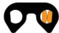
SC chain joint with "D" shaped pins
