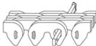
Insert longer pin through the chain.
