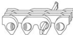
Insert longer pin through the chain.
