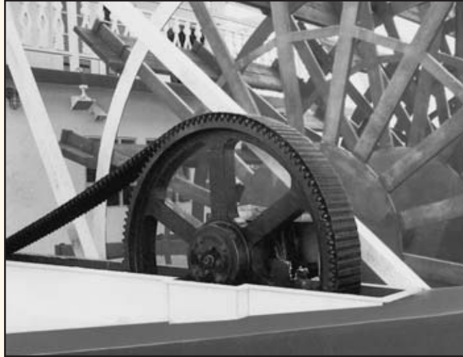
Paddle wheel drive on a large river boat
