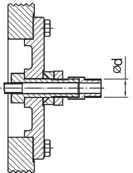
Cooling Coil Connections
